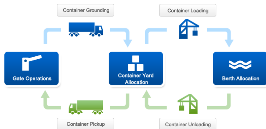
Figure 7-1 Main Operation Flows of Container Terminals
